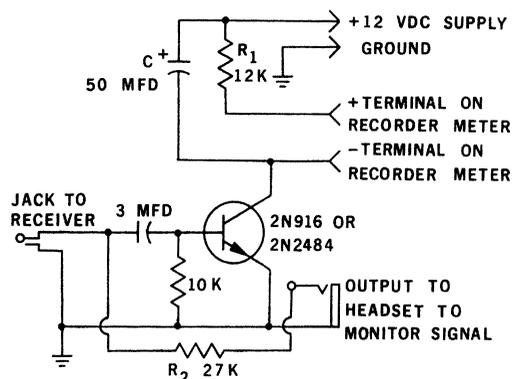
Fig. 2. Schematic diagram of the signal conditioner.
