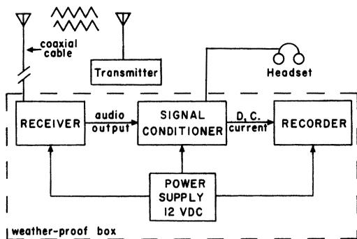
Fig. 1. Block diagram of a radio transmitter and the recorder system.
