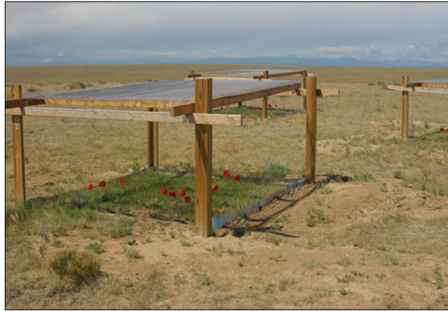
Figure 4. Example of the style of rain-out shelter proposed for the CDE to test the effects of drought in grasslands (corresponding map location in Figure 3: US [12]).
